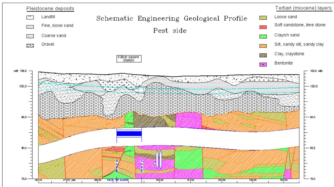
Figure 3. Variegated engineering-geological longitudinal section at Pest-side
