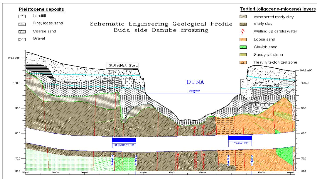
Figure 2. Schematic engineering-geological profile, Buda-side and Danube-crossing
