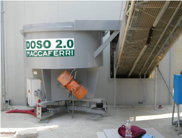
Fig. 2 Standard installed drum dosage system adding steel fibres on the conveyor belt
