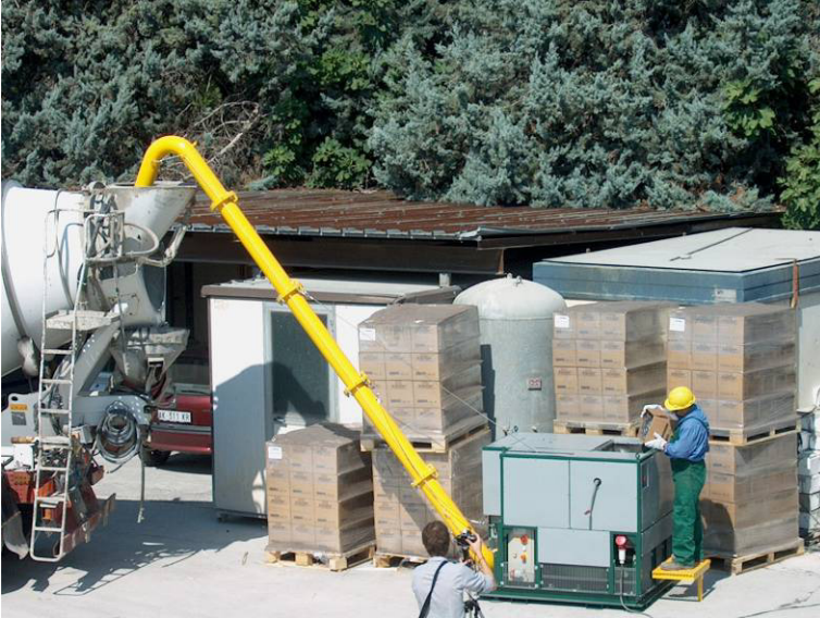
Fig. 1 Pneumatic mobile batching system for steel fibres
