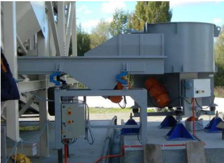
Fig. 3 Weighing vibration unit as reach extension for the standard dosage machine (Hobson Bay sewer tunnel project, Auckland)
