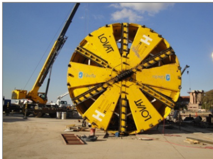
Figure 3. The cutting wheel of a LOVAT EPB used for the Hydraulic tunnel “Arroyo Maldonado”.
