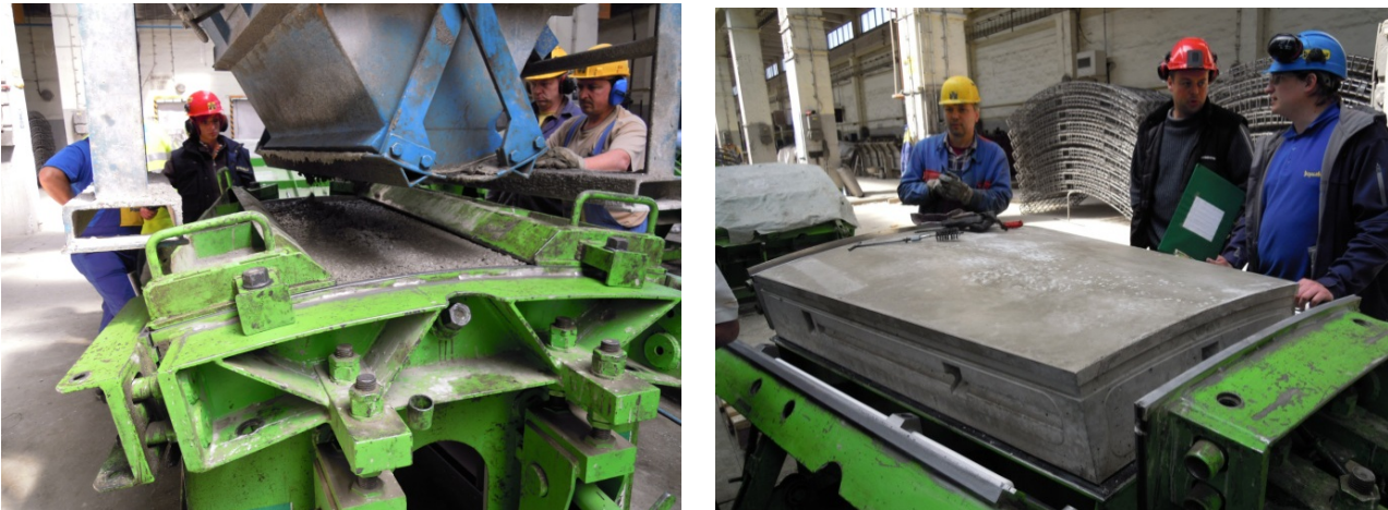
Fig. 4 Casting (left) and demoulding (right) of SFRC key segment
