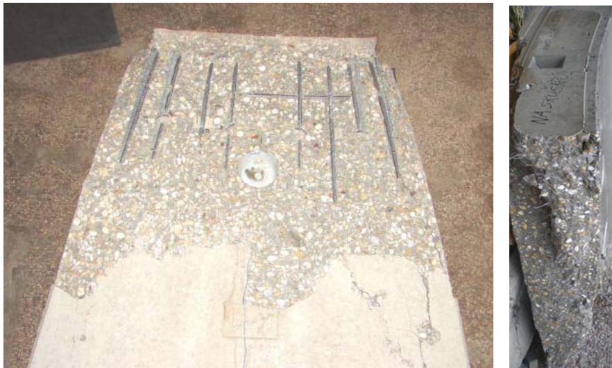
Fig. 10 Comparison of damaged key segments after reaching their capacity: (RC key segment – left, SFRC segment - right)
