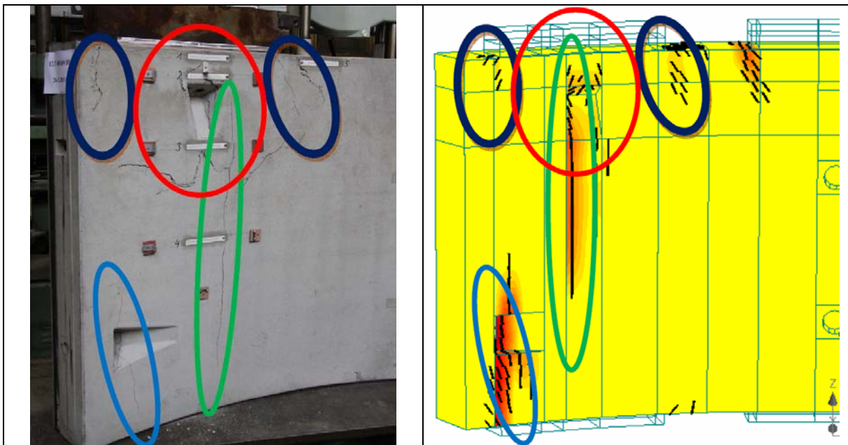
Fig. 12 Result of testing and result of modelling of RC segment in ATENA – comparison location of cracks
