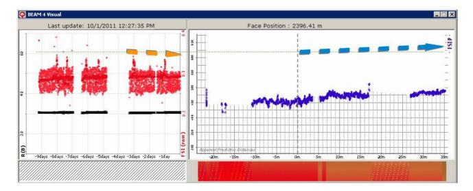
Smooth changes in rock or ground, e.g. due to gradually widening of pore spaces with waterbearing and increasing permeability, appear as linear increase or decrease of CI/IP levels (s. case above: detail of BEAM4 Visual real-time display).
