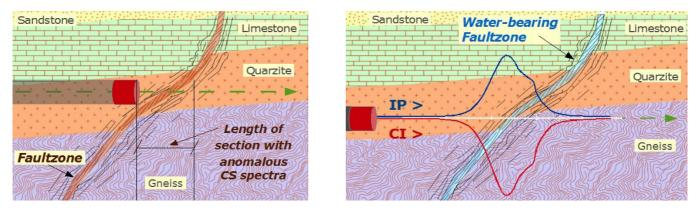
BEAM4 Integral Method – Geoelectrical Profiling along Tunnel Axis for Geology Prediction
