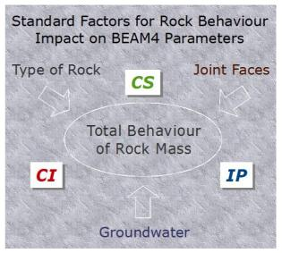
Widths of fault zones and positions of ground changes of geotechnical relevance can be detected by change of CS spectra, in certain cases even for unchanged CI and IP behaviours of rock.
