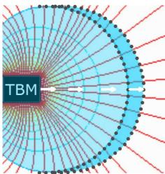
The sensitivity range of the TBM used for geoelectrical profiling is related to the tunnel diameter. Due to TBM advance, rotation-symmetric crescent-shaped differential zones develop as shown in 2D-view on left by margins of grey dotted lines for two selective TBM positions ahead, i.e. in case of homogeneous geology. Shapes and distances of 3D-differential zones differ in case of heterogeneous geology.
