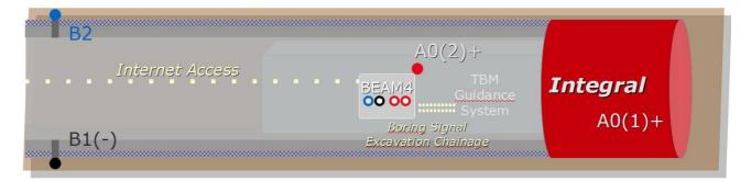
BEAM4 Scan method acquires data in two axes, i.e. parallel and vertical to the tunnel axis, whereby A0(2) is used as current sensor, A1(2) for voltage control and A2 for guard current feed (see below).
