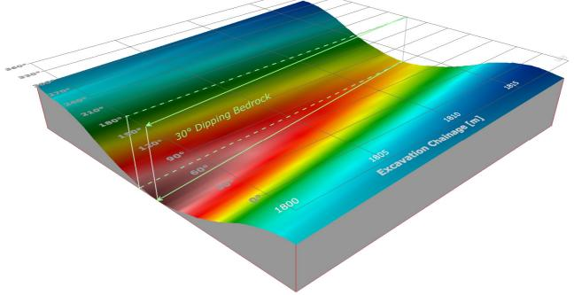
*BEAM4 Scan – Geological Prospection with two or more Focused Electrodes or El. Groups* If two or more electrodes or electrode groups are used, obstacles within the tunnel contour like karst cavities or e.g. UXO etc. can be detected by determination of different angle widths of distortion of parameter amplitudes (s. charts below with two different tool group orbits (green) and areas of amplitude distortion marked in orange).
