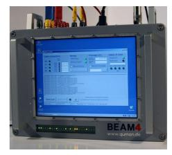
BEAM4 Scan enables to identify stratification and detection of obstacles in or nearby the tunnel contour ahead.
