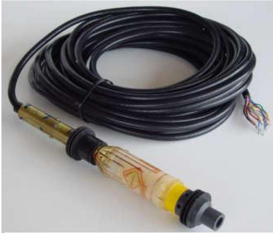
Fig. 1: CSIRO HI-cell before installation
