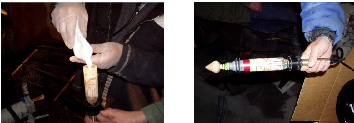
Fig. 3.: Filling the prepared adhesive into the CSIRO HI-cell (left) and the assembled cell prepared for installation (right)
