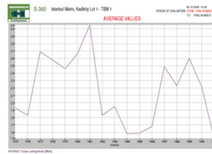
The decrease of torque due of stalling of disc cutters in blocky ground.
