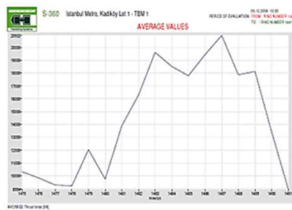
The increase of thrust force due to stalling of disc cutters in blocky ground.
