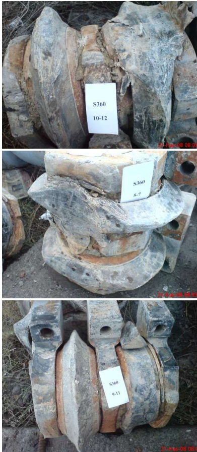
Failure of discs between 1480-1491 rings due a fault zone
