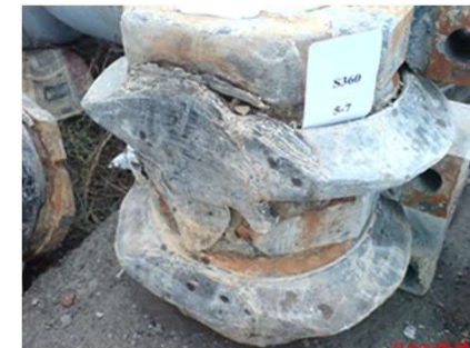
Figure. The wear of twin disc cutter due of stalling disc cutter in blocky ground.
